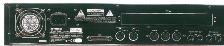
The large blanking panel on the A5000 can be used to host either the AIEB1 I/O expansion board or a forthcoming mLAN interface.
