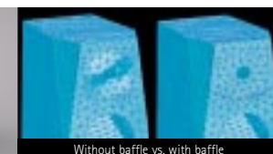
The diecast aluminium tweeter plate is very effective in damping the vibrations that occur during high frequency output.
