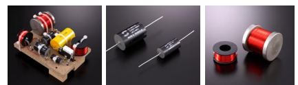
Woofer crossover network (left), Solen metalized polypropylene capacitors (centre) and large iron-core coil (right)
