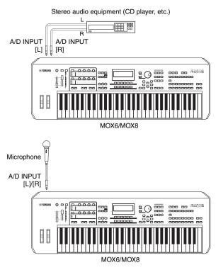
**NOTE** A standard dynamic microphone is recommended. (This instrument does not support phantom-powered condenser microphones.)
