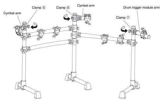
**5.** Loosen the bolts on the following seven clamps ((1)) and rotate the clamps, and then tighten the bolts again so they are secure.
