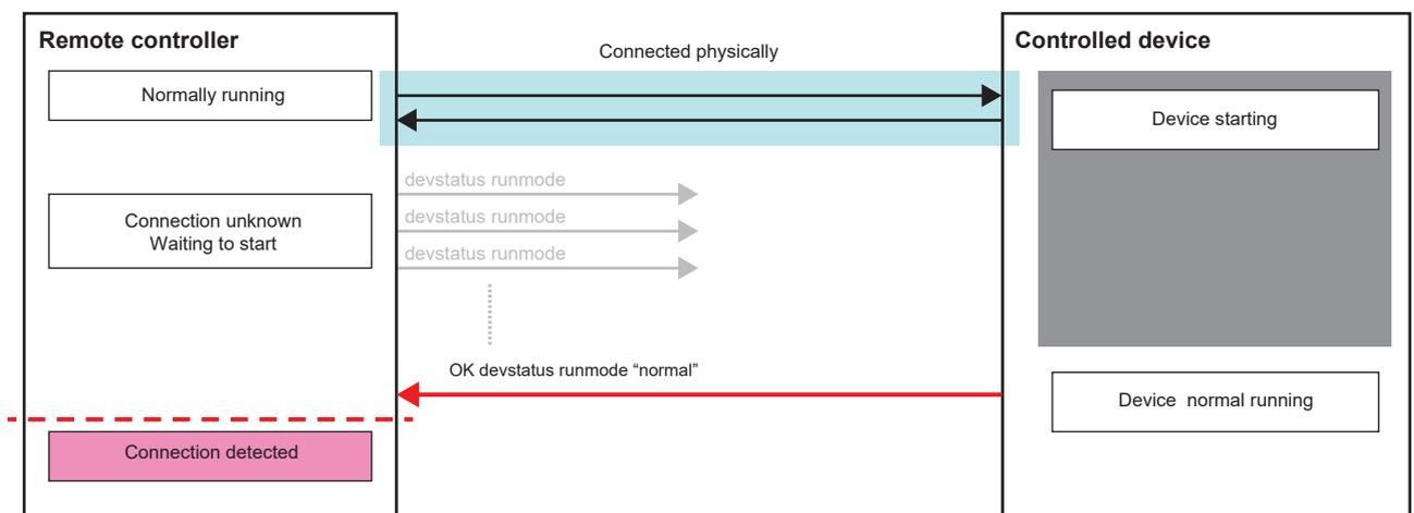
Example when the controlled device starts earlier than the controller
