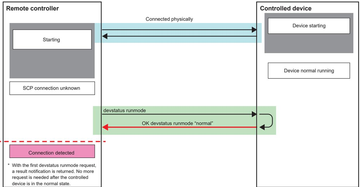
The controller can recognize that the controlled device is ready to receive commands when there is response for "devstatus runmode" command.
