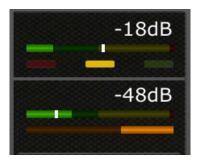
Dynamics 1 is displayed at the top of the thumbnail with Dynamics 2 at the bottom. (Output channels have only Dynamics 1.)
